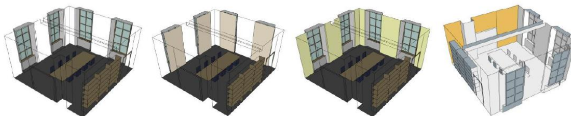
Figure 5. Simulated alternatives room A (from left to right): current situation; curtains in front of the windows (Variant 1); curtains, wall absorbers or acoustic plaster (Variant 2); wall absorption and thick carpet (Variant 3).
